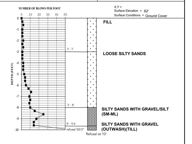
Note: Soil profile is inferred from CPT results. Subsrface conditions were not observed directly during DCP testing.
