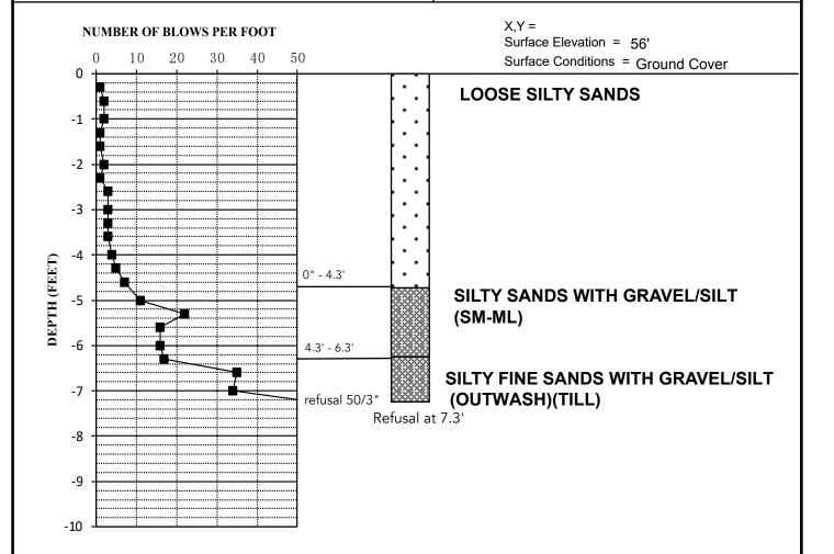
Note: Soil profile is inferred from CPT results. Subsrface conditions were not observed directly during DCP testing.
