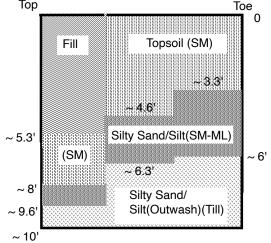
slope. The soil was dry, crumbly when disturbed, and loose in situ. However, the fill soils were encountered in DCP#3 at top of slope that is ~5 feet way from foundation of detached garage to a depth of approximately 5.3 feet below the ground surface. We interpret the existing fill as being placed during the construction of the existing detached garage.
